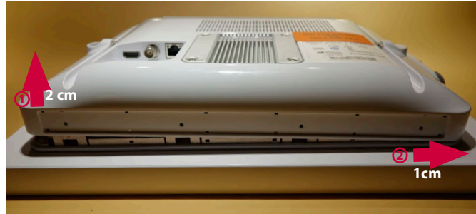
Figure 9 Carefully pull the back casing upwards and slide it slightly to the right
