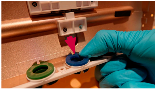
Figure 20 Remove the damaged colour ring
