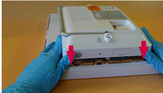
Figure 31 Place the back casing, continued
