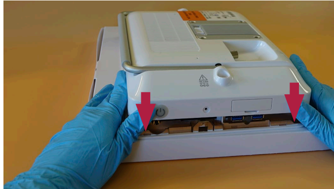
Figur 31 Anbring bagbeklædningen, fortsat
