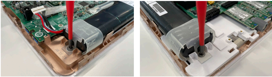
Figure 16 Unscrew screws on both sides of the battery
