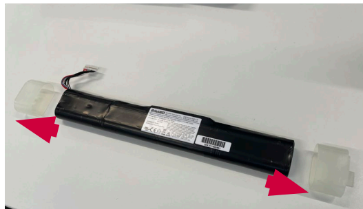
Figure 17 Carefully remove the battery caps
