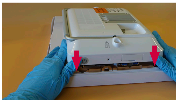
Figur 36 Anbring bagbeklædningen, fortsat
