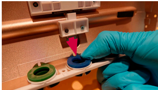
Figure 25 Remove the damaged colour ring
