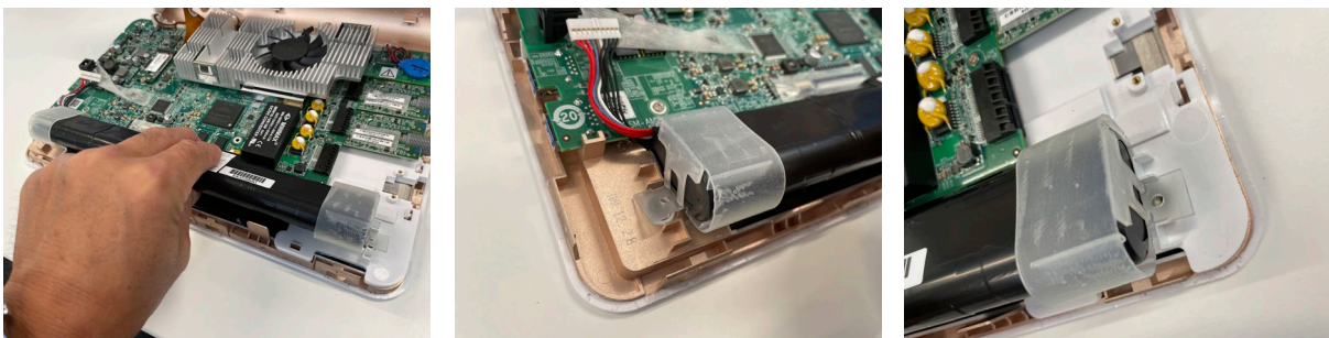
Figure 19 Place the battery with battery caps back on the device
