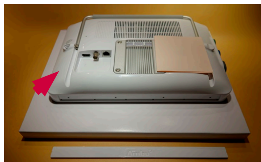
Figure 8 Place the displaying unit facing down
